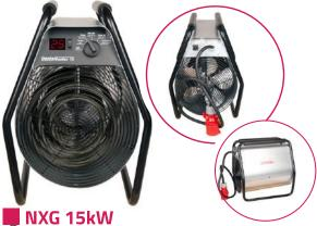
professional quality / 15kW heat output / 2 power levels + ventilator mode / adjustable room thermostat / air flow 2200m³/h / power supply 3x400V/50Hz / power cord 1,5m / 5 pin male plug / 99h ON/OFF timer
