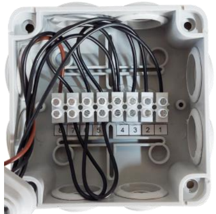
Fig. 8 p.2 Control box connectors with wires.
